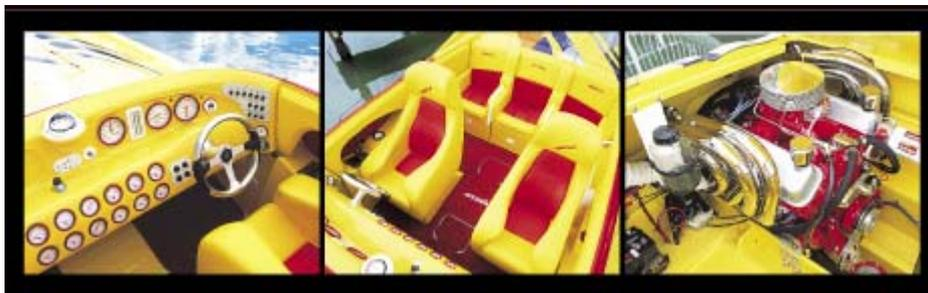
**From left:** The tach, speedo, compass and trim indicator were mounted nice and high, and all peripheral gauges came in their own recesses. In the cockpit, Hustler installed form-fitting bolsters for safety and comfort. Under the hatch, there were two naturally aspirated 725-horsepower Cobra big-blocks.
