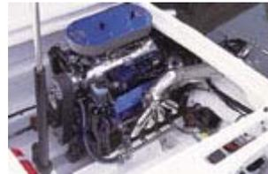
**From left:** Hustler's 377 Talon has a wraparound dash with all the instrumentation from Gaffrig. In this catamaran, the cabin is accessed by flipping up the center seat of the rear bench. Under the hatch, Hustler went with twin Keith Eickert 675-hp engines, good for 122.7 mph.
